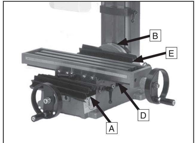
**Figure 31.** Points of lubrication.
