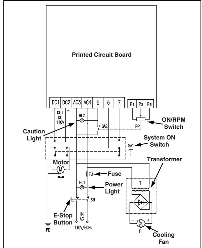
Figure 38. G8689 Wiring diagram.
