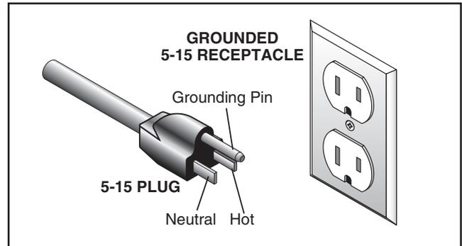
**Figure 2.** Typical 5-15 plug and receptacle.
