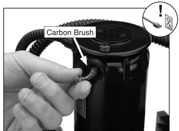
Figure 34. Carbon brush removal.
