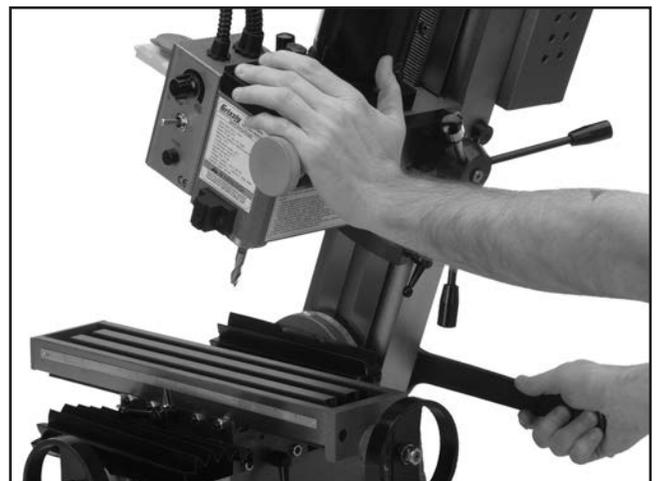
**Figure 16.** Supporting head during positioning.
