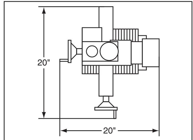
**Figure 6.** Working clearances.
