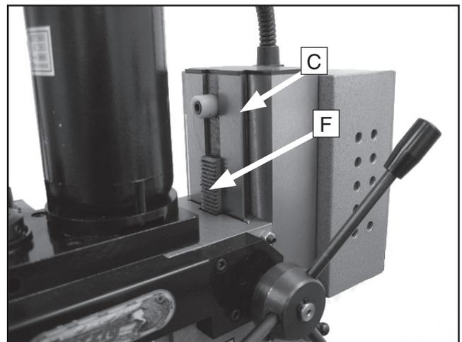
**Figure 32.** Upper column lubrication points.
