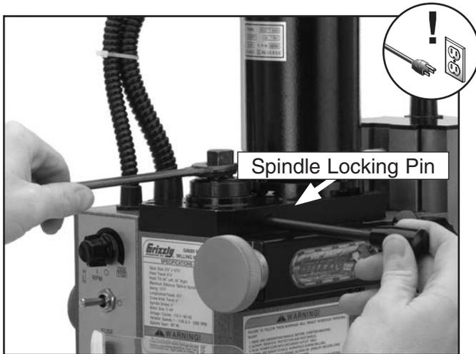
Figure 7. Loosening the drawbar.
